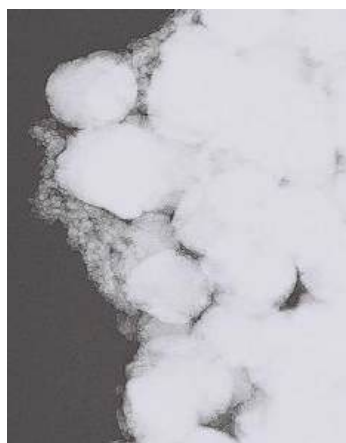
Figure 3 :TEM micrograph of an allophanic soil (the micrograph width is 600nm).
