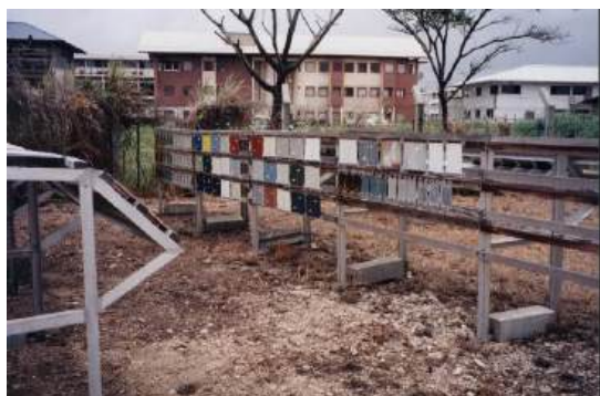
Figure 1 : stand of exposure located near the sea in Cayenne, French Guiana
